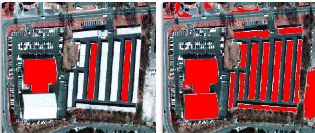
Figure 2: Left – analyst's training sample of buildings (an impervious surface class). Right – classified land cover feature of the building.
