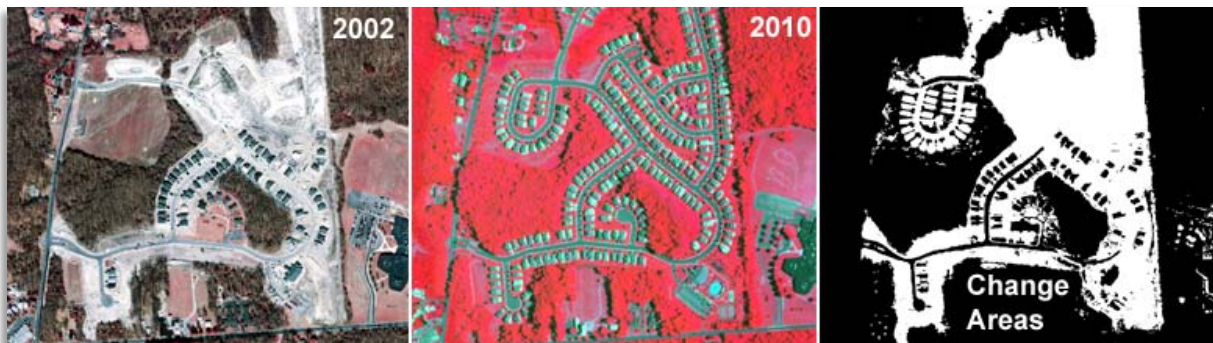
Figure 4: Binary change layer (right) created from digital change detection between 2002 and 2010 imagery.
